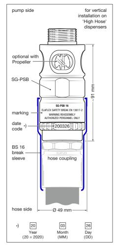
to **SG-PSB** inlet. For NPT threads do not use Teflon tape but pipe sealant on threaded connections. Check the whole system for tightness.
